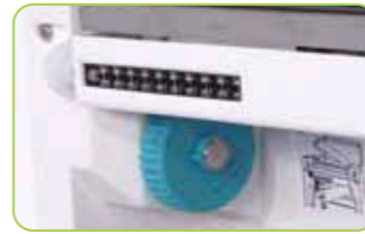
See-through sensor (Auto Detection)
